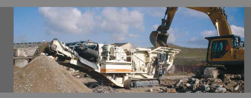
**Voladuras y Demoliciones** performs the recycling of stone materials of the demolition (concrete, ceramics and masonry) or from the excavations using portable groups of crushing machines and classification of track-mounted screening plant.
